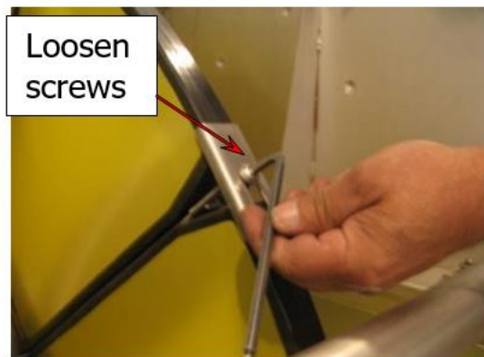
Fig. 31: Loosening a screw rails
