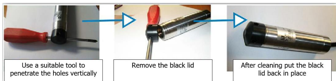
Fig. 28: Correct cleaning of a pressure probe
