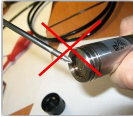
Fig. 29: Incorrect cleaning of the probe
