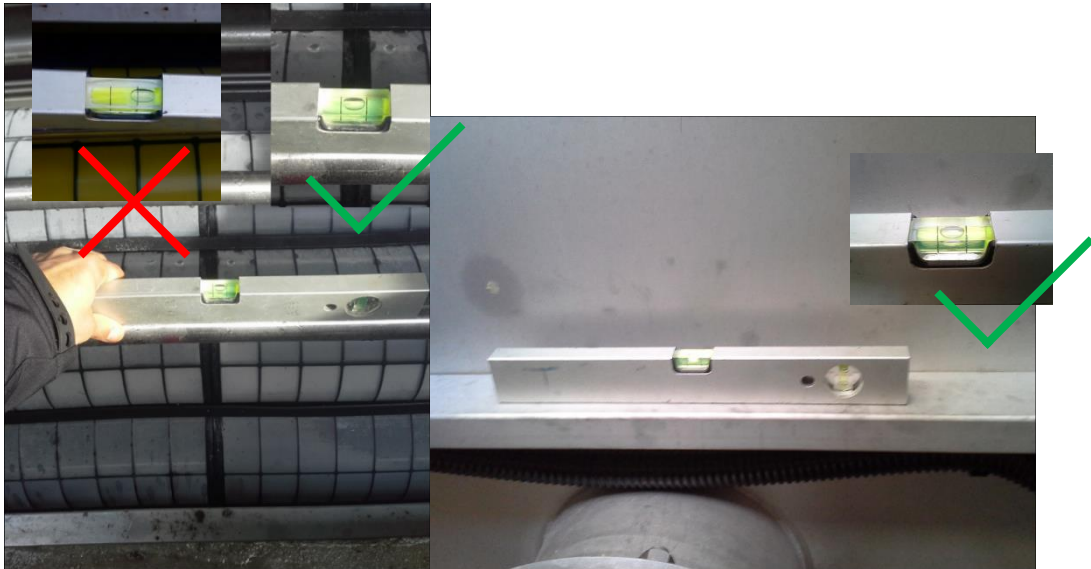
Fig. 11 Checking the horizontal position of the unit (on the shaft, from the side)
