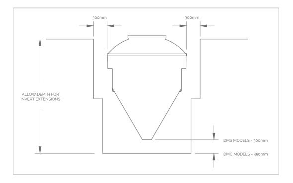
A square stepped excavation may be used due to the physical shape of the Diamond plant. Allow adequate clearance for all pipes and any other connections to the unit.
