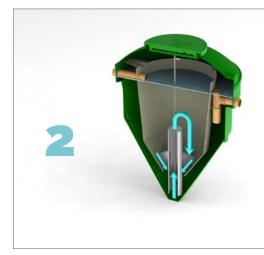
The draft tube enables the solids to be drawn back up into the central aeration chamber and re-circulated through the treatment process.
