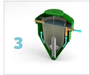
The treated liquid then exits through the dip pipe and is discharged safely in to the environment, meeting the required consent standard.
