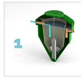
The wastewater flows into the main tank and enters directly into the bio-chamber.
