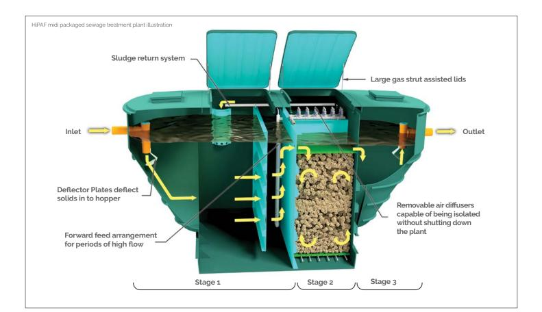
**Primary settlement -** unique forward-feed arrangement uses an airlift to deposit wastewater into the biological treatment stage, which keeps peak flows from entering the system and prevents hydraulic surges.
