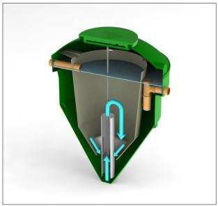
2: The draft tube enables the solids to be drawn back up into the central aeration chamber and re-circulated through the treatment process.
